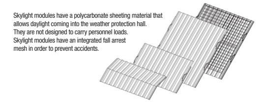
Static calculations are existing for all span widths, which are mentioned in the guide of the manufacturer for the erection and use of the modular roof system.
